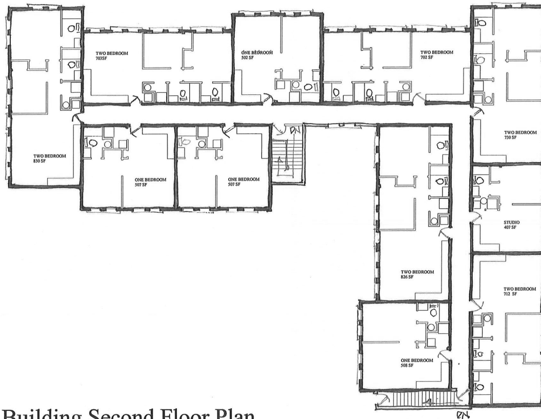
1 Proposed Building Second Floor Plan SCALE: 1/16" = 1'-0"
